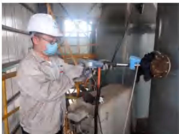
焚烧炉废气采样
